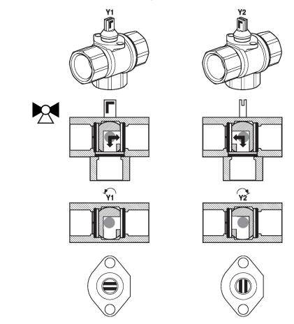
At the actuator the end stop clip has to be removed in order to get the angle of rotation of 90°, Flow setting which is needed for the change-over functionality.
